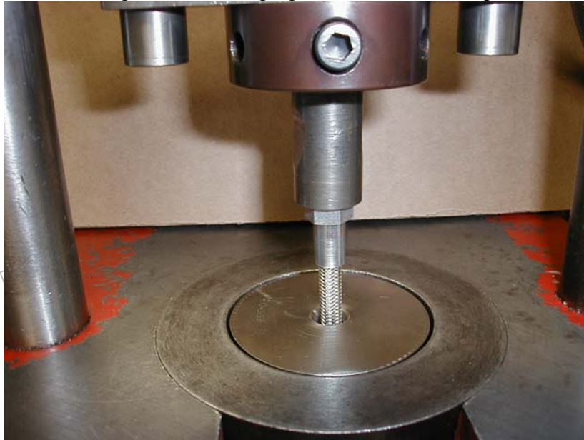
Figure #10: Swaging of Two Piece Fitting
