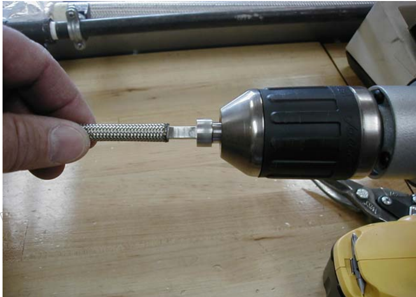
Figure #3: One Piece Fitting Installation Fixture
