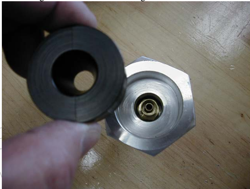
Figure #3: One Piece Fitting Installation Fixture
