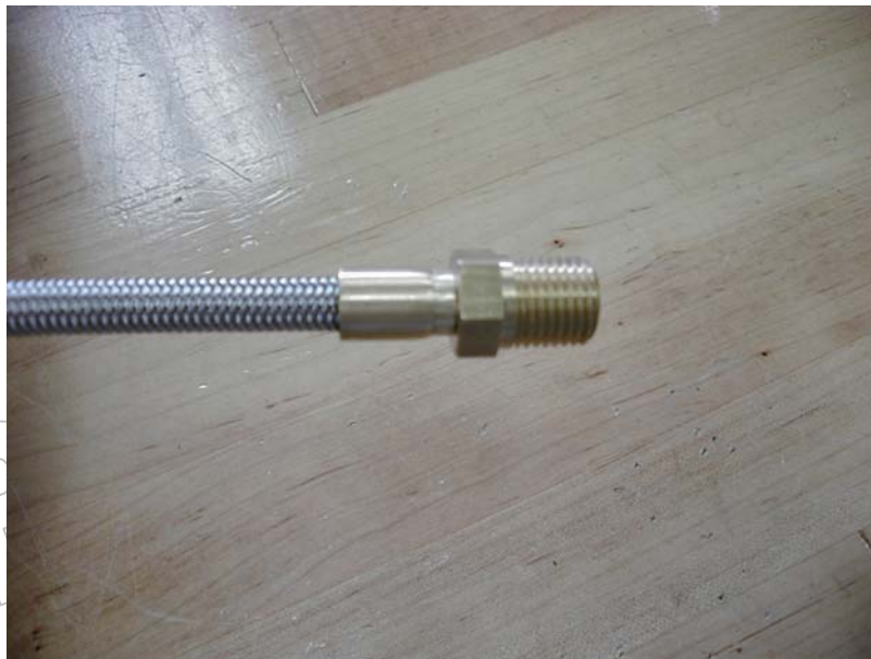
Figure #6: Swaging of One Piece Fitting
