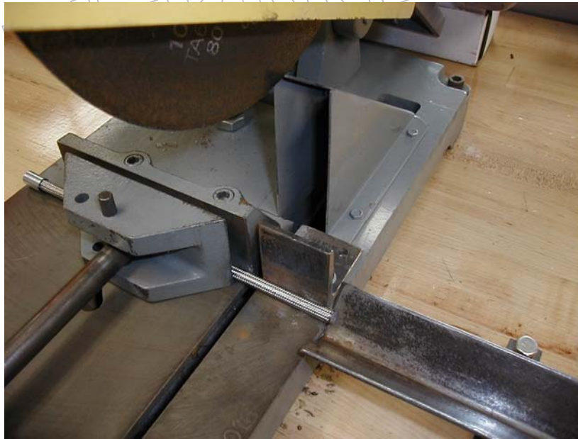
Figure #1: Hose Cut-off – Abrasive Wheel
