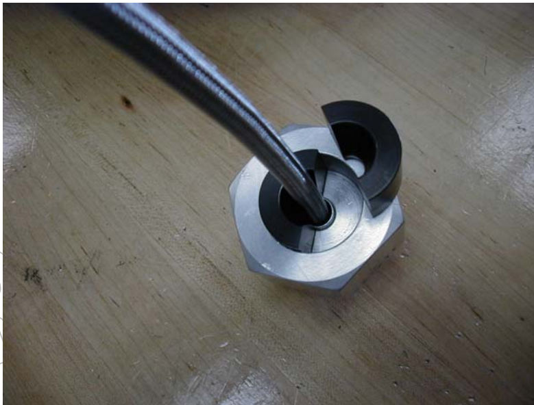
Figure #8: Hose Expansion – Two Piece Fitting
