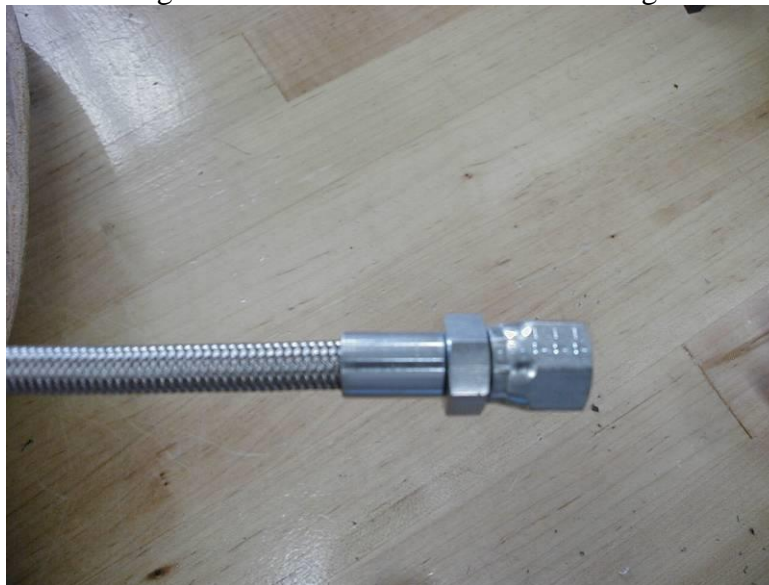
Figure #9: Assembled Two Piece Fitting
