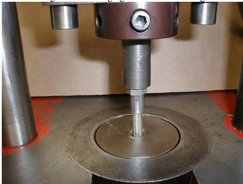
Figure #10: Swaging of Two Piece Fitting
